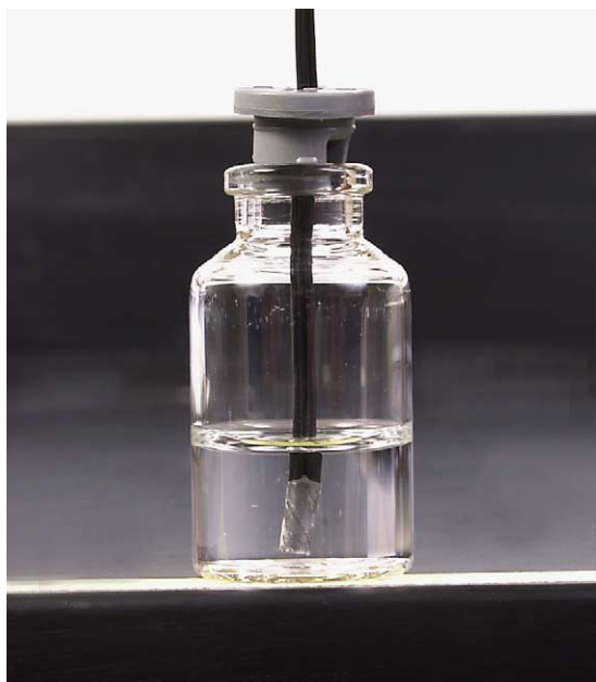
Fig. 2. Location of the thermistor probe inside a product vial.
